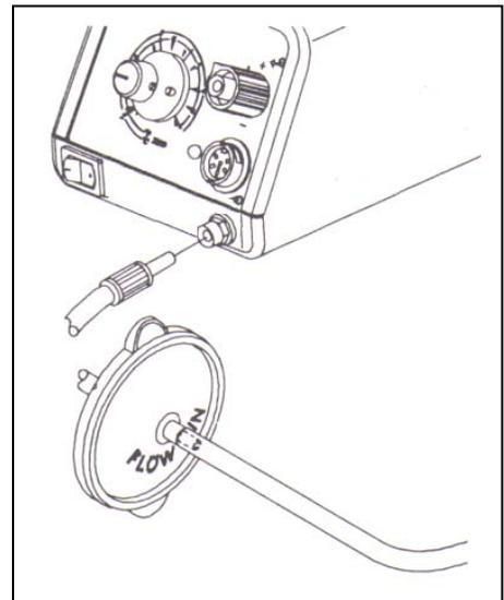
3. When using air pressure, and/or utilizing multiple air handpieces, PACE recommends the use of the following set up procedure which utilizes additional quick connect hose mount fittings. An assortment of quick connect air fittings are supplied with each additional air handpiece.
