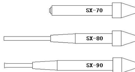
For optimal thermal transfer and performance, always use SX-90 tips with SX-90 handpieces and heater assemblies.
